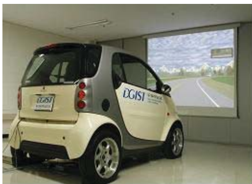
Fig. 3 The DGIST driving simulator
